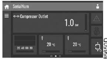
Typical display when compressor is stopped by shutdown
