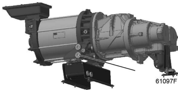
Oil drain plugs on compressor elements, gearbox and drive motor
